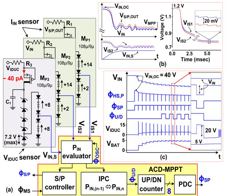
Fig. 3. Schematic of the ACD-MPPT controller.
