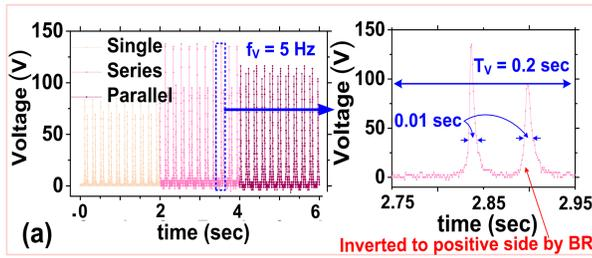
Fig. 1 shows the home made TENG pair, which is assembled using Si-rubber and Aluminum (Al) as negative and positive materials, respectively. Note that: the open-circuit voltage of TENG only exists during a short-time [1] of 0.02 sec (excitation frequency: 5 Hz), which corresponds to around 10% of the excitation frequency.
